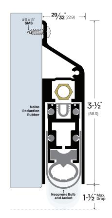
This product may be used to restore lost fire ratings due to excessive gaps at the bottom of the door up to 1-1/2 when installed per NFPA 80.
