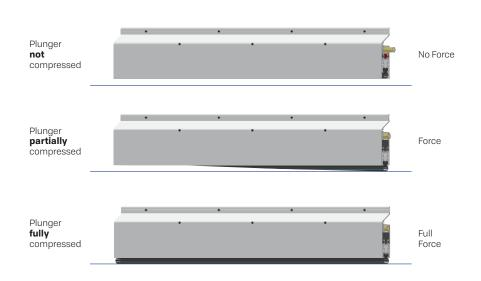
**WARNING** - Do not pull on the insert, rubber, or any components. Overextending the insert to a point lower than designed will result in binding of the unit and the inability of the insert to retract properly back into the housing Any tampering will damage the mechanism, render the seal ineffective and void the warranty.
